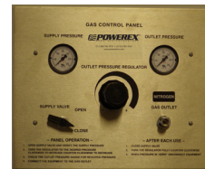
Gas Control Panel
