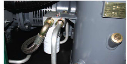
Lubricant filter assembly features a spin-on, full-flow, 12 \mu , high-efficiency element
