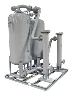
The HR / HB Series dryers are designed to be a complete air treatment solution sized for low pressure drop and performance, outfitted with standard equipment to include an oil removal 0.01 micron coalescing pre-filter, desiccant dryer for moisture removal, and a 1 micron particulate after filter in one complete package. Standard differential pressure indicators on each filter with pre-filter automatic drain all mounted to a rugged industrial steel base to enable a solidly anchored system.
