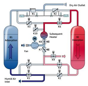
The air flow from the fan passes through the valves **K8** and **K6** to the desorbing adsorption vessel **B2**. The moisture absorbed by the desiccant evaporates and is routed by the blown-air flow from the fan through the valves **K4** and **K9** into the atmosphere.
