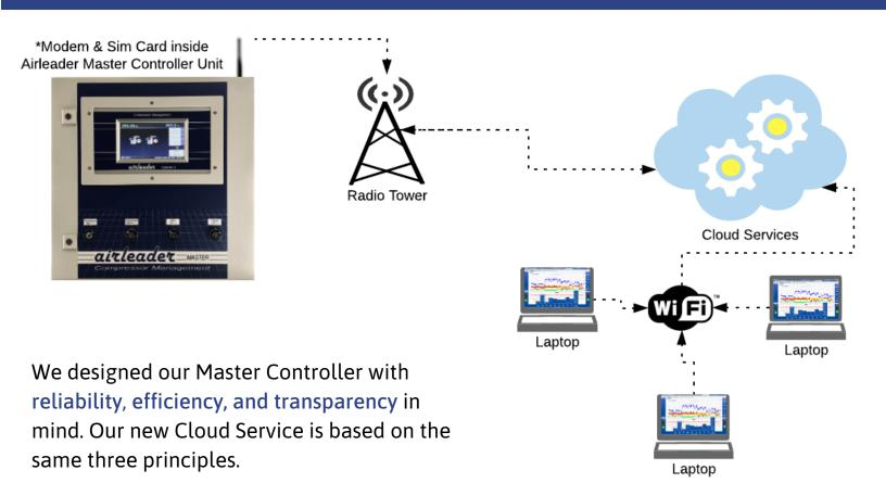
The Master Controller records all compressor data in 100% reliable, one second intervals. Information is stored in the memory of the Master Controller as well as in the Cloud. Data is continuously uploaded to the cloud and is backed up every 20 minutes to ensure the data can be viewed from both sources in case the connection is interrupted. This reliability is unmatched in the industry.
