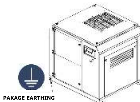
Figure 5. Earthing line of compressor
